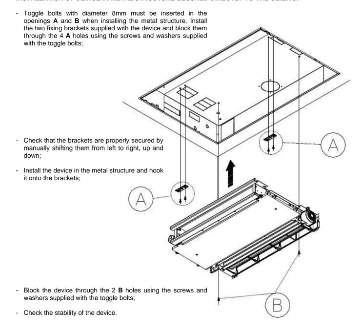
INSTALLATION OF DEVICE IN METAL STRUCTURE SECURED USING ANCHORS DETACHED FROM THE CEILING:
